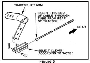
Lower tractor's attachment lift handle. Slip end of lift cable into slot on clevis (Fig. 5). Attach clevis to lowest hole of tractor lift arm with clevis pin and 1/1 6 x 1/2" potter Pin.- Reinstall seat pan and seat.
