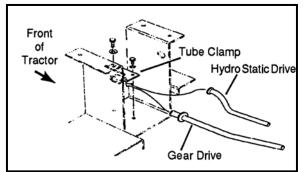
FIG. 1 Cable Tube and Clamp
